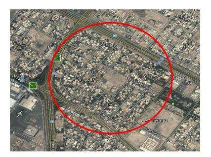
This 100 ha area was developed for national housing and the project was an upgrade to provide storm drainage, sewage and street lighting services to approx. 10 kms of suburban streets along with sidewalks, etc.
